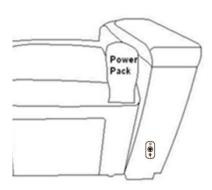
Step2: Slide back receivers into steel mechanism posts in the base of the left hand facing electric seat, and then press both sides of the back firmly into place to ensure the back automatically locks in place.
