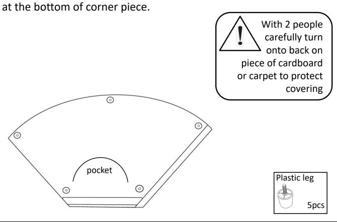
Step7: Take out the 5 plastic legs, then screw them into holes at the bottom of corner piece.
